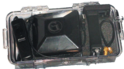
▲ COMPLETE SURVEY SET including GNSS receiver, antenna, battery and cables, fits in a small handheld plastic case.
