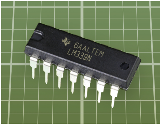
Figure 6-6. The LM339 quad comparator chip, shown here, was introduced long ago but remains widely used.
