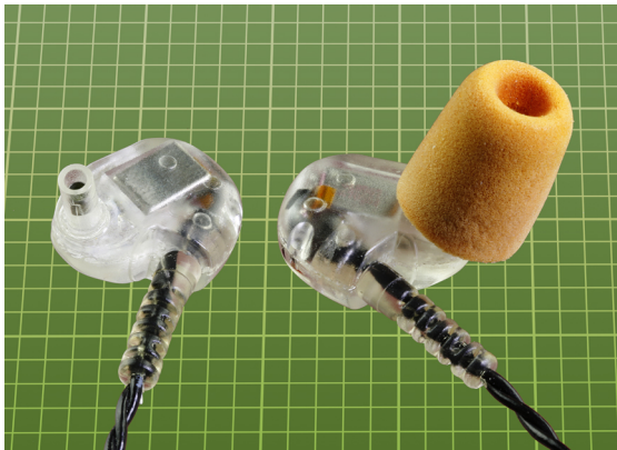
Figure 29-7. A pair of in-ear headphones, supplied with disposable foam plugs that conform flexibly with the ear canal. The headphone on the left is shown with its plug removed.
