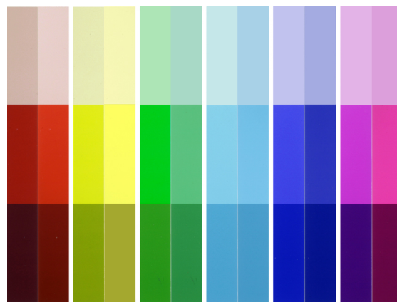
Figure 23-9. A range of six fully saturated colors, with lighter and darker shades added above and below, photographed first with “daylight spectrum” LEDs and then with halogen lights, after which the two sets of colors were paired for easy comparison. The LED version is on the left in each pair.
