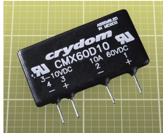
Figure 4-3. A solid-state relay capable of switching up to 10A. Its lower internal resistance results in less waste heat and enables a smaller package. See text for a detailed description.
