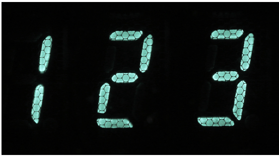
Figure 25-3. Three digits from the previous figure, showing the grid that controls their illumination.
