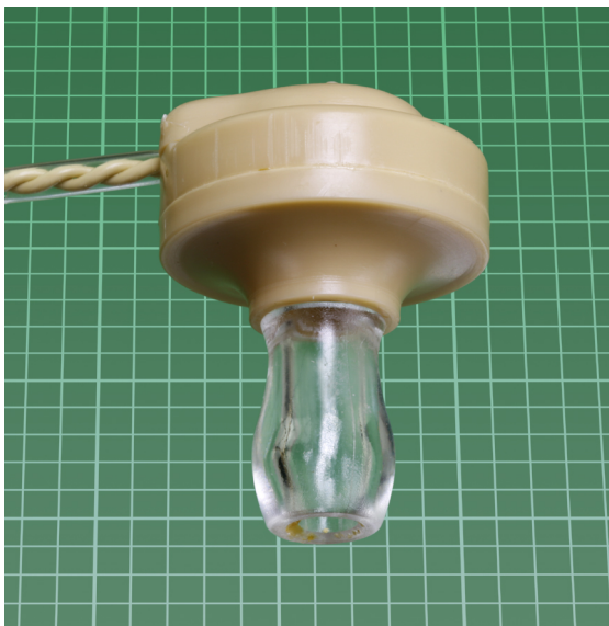
Figure 29-8. A vintage earphone of the type suitable for use with a crystal-set radio.
