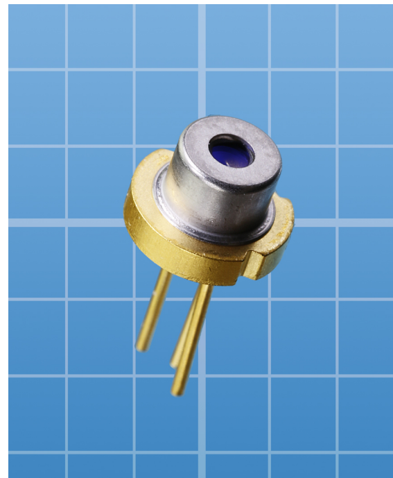
Figure 21-4. Lite-On 505T laser diode that emits light at 650nm. Power consumption 5mW at 2.6VDC. As indicated by the graph squares, this component is only about 0.2" in diameter.
