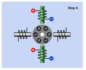
**Figure 25-12.** The bipolar stepper motor after taking its third step. When the rotor responds to the new pattern of magnetic fields, its orientation will be functionally identical with that shown in the first step.
