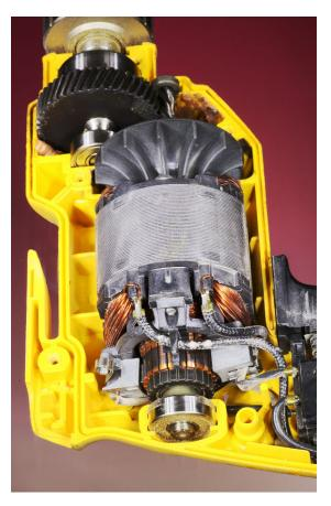
**Figure 23-12.** A motor in a corded electric drill uses coils in a brushed rotor to enable variable speed output. In most AC motors, the speed is not adjustable and the rotor does not make any electrical connection with the rest of the motor.
