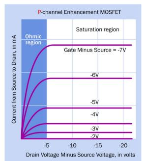
**Figure 29-19.** Current flow through an enhancementtype, P-channel MOSFET.
