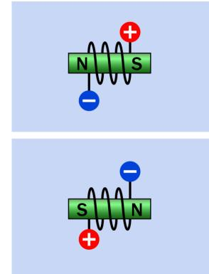
**Figure 25-3.** In a bipolar motor, the magnetic field generated by each stator coil is reversed simply by reversing the current through the coil.
