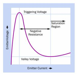
**Figure 27-5.** Response curve of a unijunction transistor (UJT). When positive potential at the emitter reaches the triggering voltage, internal resistance drops radically and the component goes through a phase known as "negative resistance" as current increases.
