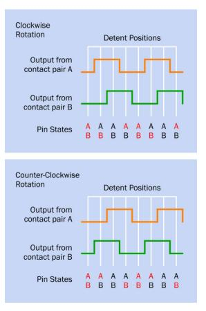
**Figure 8-2.** Hypothetical outputs from a rotational encoder, assuming that the common terminals of the contact pairs are connected to negative ground. A high pulse in the graphical representation therefore indicates that the contact pair is grounded. The number of detents relative to the number of pulses per rotation varies from one type of encoder to another.
