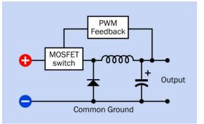
Figure 17-3. Basic topology of a buck-type DC-DC converter.
