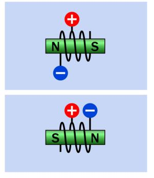
**Figure 25-4.** The magnetic field of this coil is reversed by applying positive voltage constantly to a center tap and grounding one end of the coil or the other.
