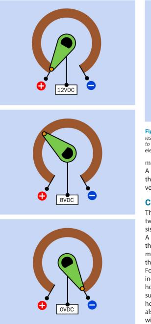
Figure 11-3. Inside a potentiometer. See text for details.
