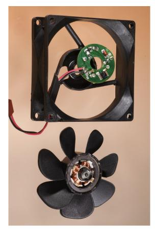
**Figure 22-10.** A typical brushless DC cooling fan uses stationary coils, with permanent magnets rotating around them.
