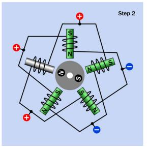
**Figure 25-18.** A multiphase stepper motor. By applying voltage in the pattern shown, only one coil is not energized during each step. This enables high torque compared with the size of the motor.
