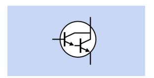
**Figure 28-9.** When a Darlington pair is embedded in a single transistor-like package, it may be represented by this schematic symbol. The leads attached to the package can be used as if they are the emitter, base, and collector of a single NPN transistor.
