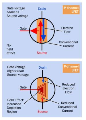
**Figure 29-5.** At top, conventional current flows freely from source to drain through the channel of a P-doped JFET. At bottom, the higher voltage of the gate relative to the source creates a field effect that pinches off the flow of current.
