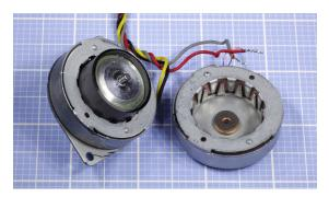
**Figure 25-6.** A two-deck stepper motor split open to reveal its rotor (left) and one of the stators (right) encircled by a coil.
