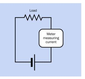
**Figure 2-11.** When measuring current using an ammeter (or a multimeter configured to measure amps), the meter must be placed in series with the battery and a load. To avoid damaging the meter, it must never be applied directly across the terminals of the battery, or in parallel with a load. Be careful to observe the polarity of the meter.
