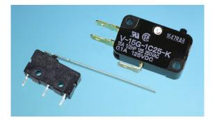
**Figure 6-4.** Two SPDT snap-action switches, also known as limit switches. The one on the right is full-size. The one on the left is miniature, with an actuator arm to provide additional leverage. The arm may be trimmed to the required length.
