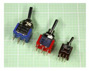
**Figure 6-10.** Three miniature toggle switches with current ratings ranging from 0.3A to 6A at 125VAC. Each small square in the background grid measures 0.1" x 0.1".
