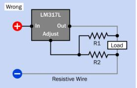
**Figure 19-7.** When the connection between an adjustableoutput voltage regulator and load components has a significant resistance (shown here as a gray "resistive wire"), R1 should always be connected as closely as possible to the pins of the regulator, as shown in the upper schematic. (Derived from schematics prepared by National Semiconductor.)
