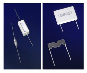
**Figure 10-13.** Two low-value resistors with their cement coatings removed to show the resistive elements.
