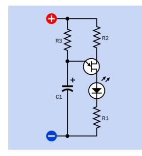
**Figure 27-8.** A basic oscillator circuit using a unijunction transistor (UJT). As the capacitor accumulates charge, the voltage on the emitter increases until it triggers the UJT, at which point the capacitor discharges through the emitter.
