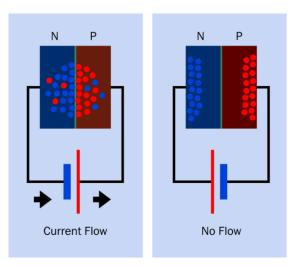
**Figure 26-4.** Inside a PN junction diode. Left: in forwardbiased mode, voltage from a battery (bottom, with plates colored for clarity) forces charges in the N and P layers toward the central junction of the diode. Current begins to flow. Right: in reverse-biased mode, charges in the N and P layers are attracted away from the central junction, which becomes a depletion region, unable to pass significant current.
