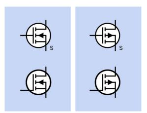
**Figure 29-13.** Schematic symbols for enhancement MOSFETs. The two on the left are functionally identical, and represent N-channel enhancement MOSFETs. The two on the right represent P-channel enhancement MOS-FETs.
