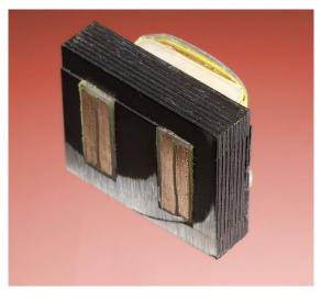
**Figure 15-8.** The small transformer from the first figure in this entry is shown sliced open to reveal its internal configuration.
