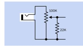
**Figure 11-11.** In this circuit, a 100K linear potentiometer is used in conjunction with a 22K resistor to create an approximately logarithmic volume control for an audio system with input coming from a mono jack socket at left.
