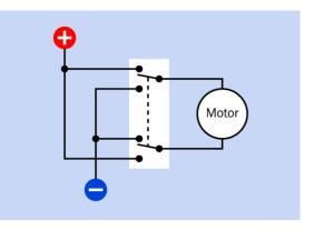
**Figure 22-13.** A DPDT switch or relay can reverse the direction of a traditional DC motor simply by swapping the polarity of the power supply.
