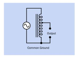
**Figure 15-10.** An autotransformer contains only one coil and core. A reduced output voltage can be obtained by tapping into the coil. A common connection prevents the output from being electrically isolated from the input.
