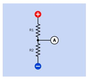
**Figure 10-20.** In a DC circuit, a pair of resistors may be placed in series to function as a voltage divider. The voltage measured at A will be lower than the supply voltage, but above ground potential.
