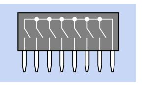
**Figure 6-18.** The interior connections of an 8-pin SIP switch incorporating a common bus.
