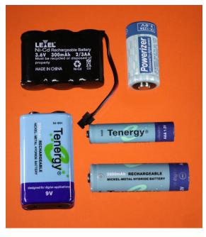
**Figure 2-9.** Top left: NiCad battery pack for a cordless phone. Top right: Lithium battery for a digital camera. The other batteries are rechargeable NiMH substitutes for everyday alkaline cells.
