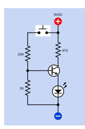
**Figure 28-6.** This simple schematic can be used to breadboard-test a transistor empirically, determining its functionality and the identities of its collector and emitter leads.
