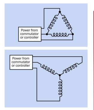
**Figure 22-5.** Coils on the rotor of a traditional DC motor may be connected in delta configuration (top) or wye configuration (bottom).
