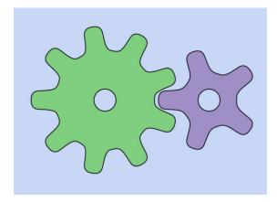
Figure 22-8. A pair of spur gears.
