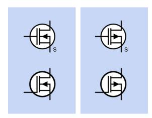
**Figure 29-12.** Schematic symbols for depletion MOS-FETs. These function similarly to JFETs. The two symbols on the left are functionally identical, and represent Nchannel depletion MOSFETs. The two symbols on the right are both widely used to represent P-channel depletion MOSFETs.
