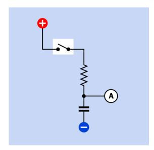
**Figure 10-19.** In an RC (resistor-capacitor) network, a resistor limits the rate of increase in potential of the capacitor, measured at A, when the switch is closed.
