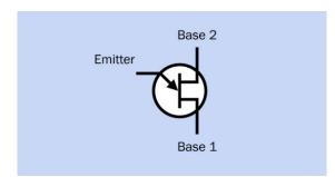
**Figure 27-1.** Schematic symbol for a unijunction transistor (UJT). Note the bent arrow. The symbol for a field-effect transistor looks similar, but has a straight arrow. The functionality of the two components is very different.
