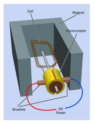
**Figure 22-1.** The simplest traditional DC motor contains these parts. The combination of coil, shaft, and commutator is the rotor. The fixed magnetic structure in which it rotates is the stator.
