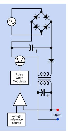
**Figure 16-4.** Greatly simplified schematic showing the principal components of a switching power supply. Note the absence of a 115VAC power transformer. The transformer that is inserted subsequently in the circuit functions in conjunction with the high switching frequency, which allows it to be very much smaller, cheaper, and lighter.
