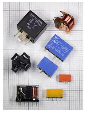
**Figure 9-4.** An assortment of small DC-powered relays. See text for details.
