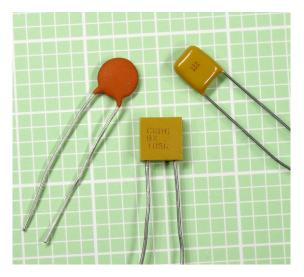
**Figure 12-7.** Generic ceramic capacitors. Left: rated for  $0.1\mu$ F at 50V. Center:  $1\mu$ F at 50V. Right:  $1\mu$ F at 50V.
