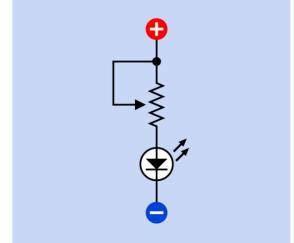
**Figure 11-4.** A potentiometer can be used to adjust a series resistance, as shown in this schematic. Tying the wiper to one of the end terminals reduces the risk of picking up electrical noise.
