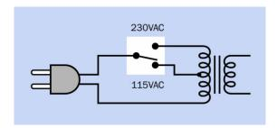
**Figure 15-5.** An international power adapter can provide a fixed output voltage by using a double-throw switch to apply 230VAC voltage across a transformer's primary winding, or 115VAC to a tapped midpoint of the primary winding.
