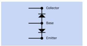
**Figure 28-5.** An NPN transistor can behave as if it contains two diodes connected as shown. Where the functions of the leads of the transistor are unknown, the base can be identified by testing for conductivity.
