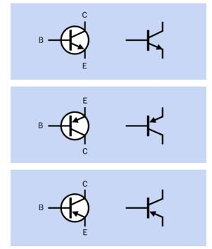
**Figure 28-1.** Symbols for an NPN transistor (top) and a PNP transistor (center and bottom). Depending on the schematic in which the symbol appears, it may be rotated or inverted. The circle may be omitted, but the function of the component remains the same.
