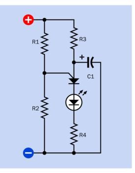
**Figure 27-9.** A basic oscillator circuit using a programmable unijunction transistor (PUT). As the capacitor accumulates charge, the voltage on the anode increases until it triggers the PUT, at which point the capacitor discharges through the anode. The gate voltage is preset by R1 and R2 to adjust the triggering voltage.
