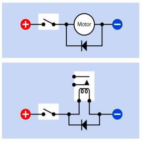
**Figure 26-15.** A rectifier diode is very often placed across a motor (top), relay (bottom), or other device with significant inductance that creates a spike of reverse voltage when switched on or off. The surge is shunted through the diode, protecting other components in the circuit.
