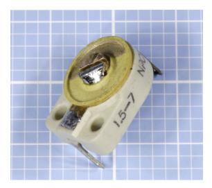
Figure 13-4. A trimmer capacitor rated 1.5pF to 7.0pF.
