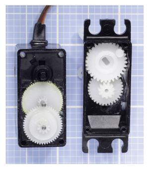
Figure 24-6. Nylon gearing inside a servo motor.
