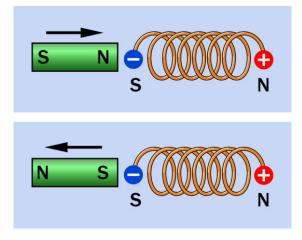
**Figure 14-8.** A permanent magnet (left) will either be drawn toward a DC-energized coil or repelled from it, depending on the polarity of the two magnetic fields.
