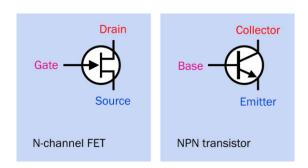
**Figure 29-1.** A comparison between schematic symbols for N-channel JFET (left) and NPN bipolar transistor (right) suggests their functional similarity as switches or amplifiers, although their behavior is markedly different.
