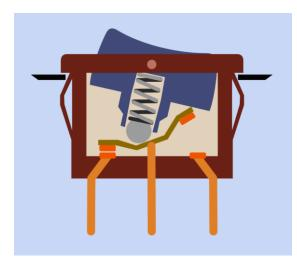
**Figure 6-7.** This sectional view of a rocker switch shows a spring-loaded ball-bearing that rolls to and fro along a rocker arm, connecting either pair of contacts when the switch is turned.
