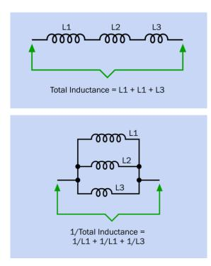
Figure 14-21. Calculating the total inductance of inductors in parallel (top) and series (bottom).
