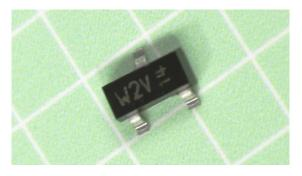
**Figure 28-12.** A surface-mount package for a Darlington pair. Each square in the background grid measures 0.1". See text for additional details.
