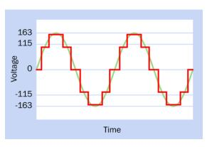
**Figure 18-4.** A secondary stream of narrower squarewave pulses can improve the fidelity of an inverter's output.
