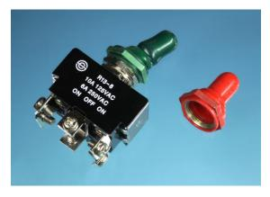
**Figure 6-14.** A rubber or vinyl boot can be used to protect a toggle switch from contamination with dirt or water. Each boot contains a nut that screws onto the threads of a toggle switch, as shown at left.
