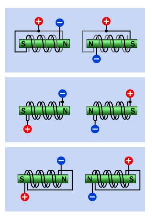
**Figure 25-17.** In a bifilar motor, two coils are wound in parallel around each stator pole and can be connected with a center tap to emulate a unipolar motor (upper diagrams), or can be energized in parallel (middle diagrams) or series (lower diagrams) to emulate a bipolar motor.
