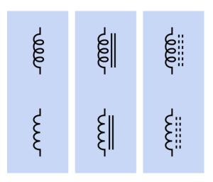
**Figure 14-1.** The coil symbol for an inductor may be drawn in two styles which are functionally identical. Line(s) beside the coil indicate a solid core. Dotted line(s) indicate a core containing metal particles.
