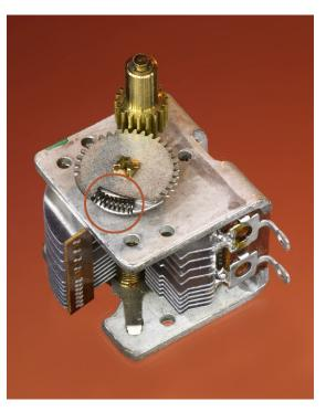
**Figure 13-3.** A "traditional style" variable capacitor of the type designed to tune radio frequencies. The spring, circled, enables anti-backlash gearing.
