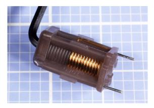
**Figure 14-12.** A variable inductor. Its inductance is adjusted via a screw thread that varies the insertion of the core in the coil. In this component the core is turned by inserting a hex wrench, as shown. It is rated from  $0.09\mu$ H to  $0.12\mu$ H.
