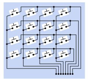
**Figure 5-11.** Buttons in a numeric keypad are usually wired as a matrix, where each button makes a connection between a unique pair of wires. This system is suitable for being polled by a microcontroller.
