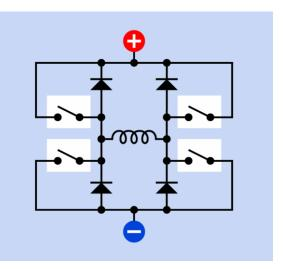
**Figure 25-19.** The H-bridge circuit must be augmented with protection diodes to guard against back-EMF created by fluctuating current in the stator coil.
