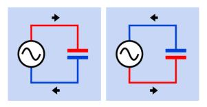
**Figure 12-4.** In the left diagram, a source of alternating current charges the upper plate of a capacitor positively and the lower plate negatively. This process entails a flow of conventional current shown by the arrows. A moment later, when the AC current flow reverses, the flow also reverses, creating the impression that the capacitor "passes" AC current.
