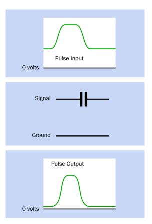
**Figure 12-20.** A coupling capacitor (typically around  $1\mu$ F) preserves DC isolation of one section of a circuit from another, while allowing a pulse to be transmitted.
