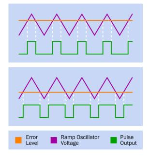
**Figure 17-2.** To achieve pulse-width modulation, an errorlevel voltage is established by comparing the output from the converter with a reference voltage. The error level, shown as an orange line, is then subtracted from the output from a ramp oscillator. The pulse width varies accordingly.
