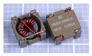
**Figure 14-16.** A larger-sized surface-mount toroidal inductor (viewed from the bottom, at left, and from the top, at right). It is rated at  $3.8\mu$ H.
