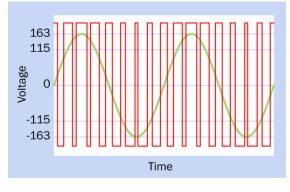
**Figure 18-5.** Pulse-width modulation adjusts the widths of pulses delivered at a high frequency. The pulse widths can be averaged to generate voltage that follows a close approximation of a sine wave.
