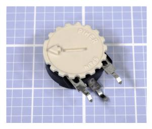
**Figure 11-9.** A trimmer potentiometer with a knurled dial to facilitate finger adjustment.
