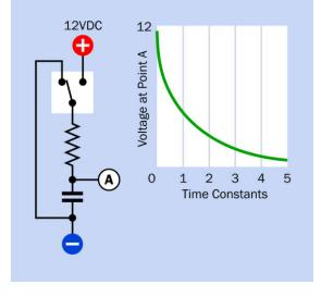
**Figure 12-3.** An RC (Resistor-Capacitor) network with a switch to control charge and discharge of a capacitor. At top, the curve gives an approximate idea of the charging behavior of the capacitor. At bottom, the curve illustrates its discharging behavior.
