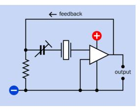
**Figure 13-7.** A trimmer capacitor in series with a crystal fine-tunes the frequency of this basic circuit using an op-amp.
