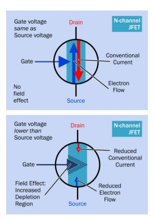
**Figure 29-4.** At top, conventional current flows freely from drain to source through the channel of an N-doped JFET. At bottom, the lowered voltage of the gate relative to the source creates a field effect that pinches off the flow of current.
