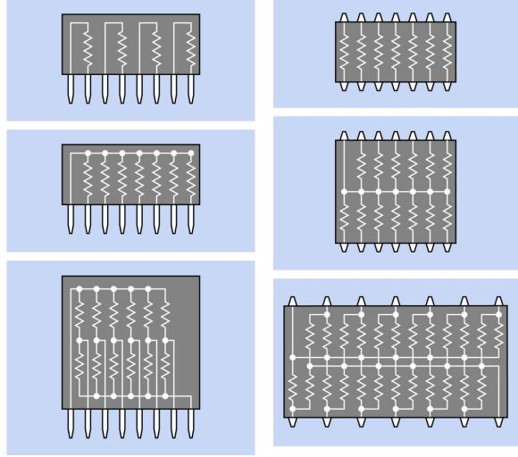
**Figure 10-4.** Multiple resistors can be embedded in a single-inline package (SIP) in a variety of formats. See text for additional details.
