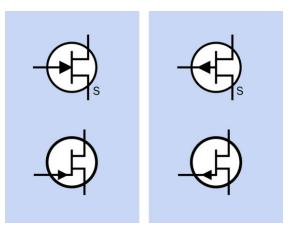
**Figure 29-3.** Schematic symbols for junction field-effect transistors (JFETs). Left: N-channel. Right: P-channel. The symbols at top and bottom on each side are functionally identical. Circles may be omitted. Letter S may be omitted from the symmetrical symbol variants, even though this creates some ambiguity.
