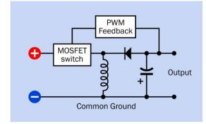
**Figure 17-5.** Basic topology of a flyback-type DC-DC converter.
