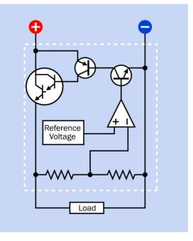
**Figure 19-3.** The fundamental internal features of a standard-type voltage regulator, including a Darlington pair, two transistors, a voltage divider, comparator, and reference voltage source, shown inside the dashed white line.
