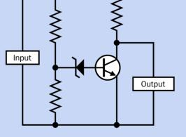
**Figure 26-23.** A Zener diode can be used in conjunction with a PNP transistor. See text for details.
