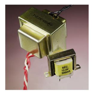
**Figure 15-1.** Two small power transformers. The one at the rear measures approximately  $1" \times 2" \times 2"$  and is rated to provide 36VAC at 0.8A. The term "sec" on the smaller unit is an abbreviation for "secondary," referring to the rating for its secondary winding.
