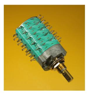
Figure 7-4. A five-pole, twelve-position rotary switch.
