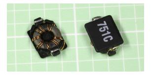
**Figure 14-14.** In a typical toroidal inductor, the coil is wrapped around a magnetic core shaped as a torus. This surface-mount component (viewed from the bottom, at left, and from the top, at right) is at the low end of the range of component sizes. It is rated at 750nH.
