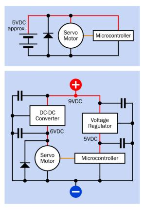
**Figure 24-7.** Two possible schematics to run a small servo motor, the upper example using battery power (for example, from four 1.2V NiMH cells) and the lower example using a 9VDC AC adapter. See text for additional explanation.
