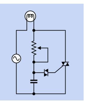
**Figure 11-10.** Typical usage of a potentiometer in conjunction with a diac, triac, and capacitor to control the brightness of an incandescent bulb, using an AC power supply. Diacs and triacs are discussed in Volume 2.
