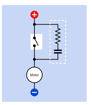
**Figure 12-24.** An RC network (outlined with a white dashed line) protects a switch that controls a high inductive load. Used in this way, the RC network is known as a snubber.
