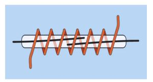
**Figure 9-7.** This simplified rendering shows a reed relay, consisting of a magnetized reed switch inside a glass or plastic pod, activated by a coil wrapped around it.
