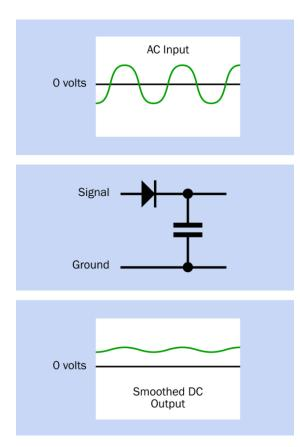
**Figure 12-23.** A capacitor of  $100\mu$ F or more smooths the upper half of an AC signal that has passed through a diode. The capacitor charges during each positive pulse and discharges to "fill the gaps" between them.
