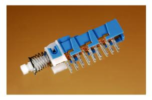
**Figure 5-9.** This 6PDT pushbutton latches and then unlatches, each time it is pressed.
