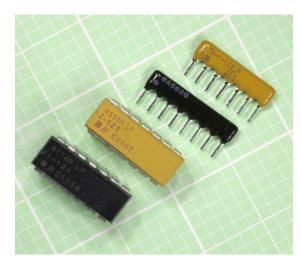
**Figure 10-6.** Resistor arrays in DIP and SIP packages. See text for values.
