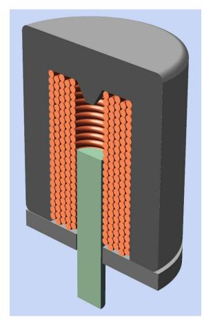
**Figure 21-3.** A simplified view of a solenoid cut in half, showing the primary parts.
