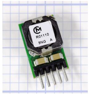
**Figure 17-8.** An adjustable DC-DC converter rated for 10A or 50W. The output voltage is determined by adding an external resistor or trimmer potentiometer. External smoothing capacitors are required, as shown in the component's datasheet.
