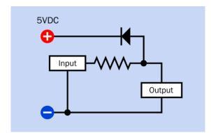
**Figure 26-17.** A clamping diode can limit output voltage in this example, to about 5.6V. If the input rises above that value relative to the common ground, the potential difference across the diode feeds the excess voltage back through it to the 5V source.
