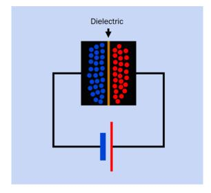
**Figure 12-2.** Because the plates of a capacitor are electrically conductive, they will become populated with positive and negative charges when connected with a DC power source. As opposite charges attract each other, they will tend to congregate on either side of the dielectric, which is an insulating layer. The battery symbol is shown here colored for clarity.
