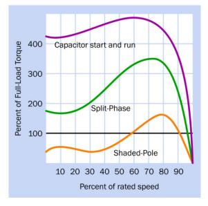
**Figure 23-10.** Approximate curves showing the relationship between speed and torque for three types of singlephase induction motor. (Graph derived from AC Induction Motor Fundamentals published by Microchip Technology Inc.)
