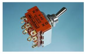
**Figure 6-12.** A 4PDT full-size toggle switch with solder terminals, capable of switching 25A at 125VAC. Four-pole switches are relatively unusual.
