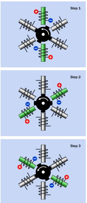
**Figure 25-2.** In a variable reluctance stepper motor, the rotor moves to minimize magnetic reluctance each time the next pair of coils is energized. At each step, the coils have been energized a moment before the rotor has had time to respond.
