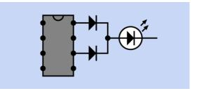
**Figure 26-18.** Two or more outputs from a logic chip or microcontroller may be coupled with diodes to power another device, such as an LED, while protecting the chip from backflow of current. The diodes form a logical OR gate.
