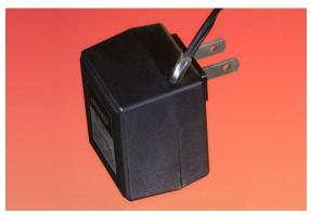
**Figure 16-2.** A simple transformer-based power supply can be encapsulated in a plastic shell, ready to plug into a power outlet. However, today this format more typically contains a switching power supply, which is usually lighter, smaller, and cheaper.
