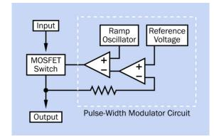
**Figure 17-1.** The heart of a DC-DC converter is a MOSFET switch, which operates at a high frequency with pulse-width modulation used to create an adjustable DC output.
