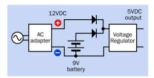
**Figure 26-16.** Two diodes with their cathodes tied together will choose automatically between an AC adapter that delivers 12VDC and an internal 9V battery.
