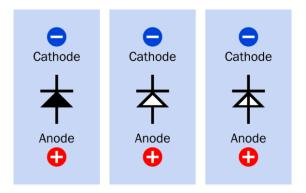
**Figure 26-1.** Commonly used schematic symbols for a generic diode. All the symbols are functionally identical. The direction of the arrow formed by the triangle indicates the direction of conventional current (from positive to negative) when the diode is forward-biased.
