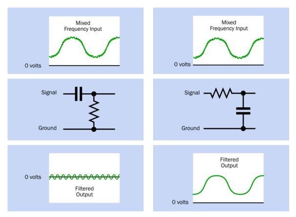
**Figure 12-21.** A small capacitor (typically  $0.1\mu$ F) can be used to create a high-pass filter, passing high frequencies while blocking low frequencies.
