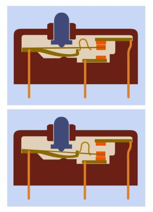
**Figure 6-5.** Top: Two contacts inside this limit switch are touching by default. Bottom: When the external button is pressed, it pushes a flexible metal strip downward until it connects with the lower contact. The inverted-U–shaped component is a spring that rests inside a cutout in the flexible strip and resists motion through the central part of its travel.
