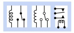
**Figure 9-2.** Commonly used schematic symbols for a SPDT relay. The symbols are functionally identical.
