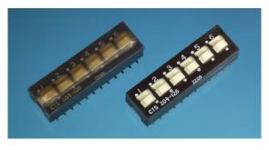
**Figure 6-17.** A SPDT surface-mount double-throw DIP switch, sold with a plastic cover (shown at left) to protect it during wave soldering. The cover has been removed at right.
