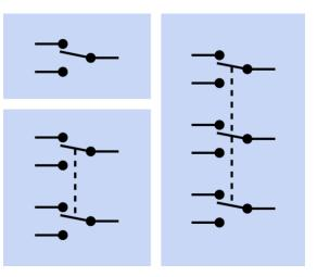
**Figure 6-3.** Schematic symbols to represent three types of double-throw switch. Top left: Single-pole. Bottom left: Double-pole. Right: Triple-pole, more commonly known as 3-pole.
