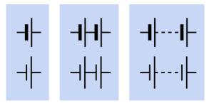
**Figure 2-2.** Schematic symbols for a battery. Each pair of symbols within a blue rectangle is functionally identical.
