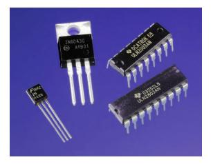
**Figure 28-10.** Various packaging options for Darlington pairs. From left to right: The 2N6426 contains a Darlington pair rated to pass up to 500mA continuous collector current. The 2N6043 is rated for 8A continuous. The ULN2003 and ULN2083 chips contain seven and eight Darlington pairs, respectively.
