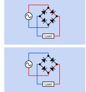
**Figure 26-9.** The basic circuit commonly used to form a bridge rectifier, with color added to indicate polarity. Wires shown in black are not passing current because diodes are blocking it. Note that the polarity at the load remains constant.
