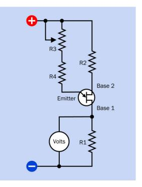
**Figure 27-6.** A test circuit for a unijunction transistor (UJT) using a volt meter to show its response as a potentiometer increases the voltage applied to its emitter.
