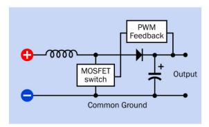
**Figure 17-4.** Basic topology of a boost-type DC-DC converter.
