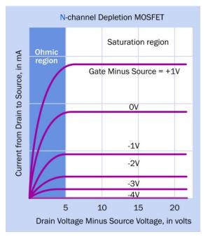
**Figure 29-16.** Current flow through a depletion-type, N-channel MOSFET.
