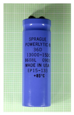
**Figure 12-11.** This 13,000µF electrolytic capacitor is larger than would be required in most everyday applications.
