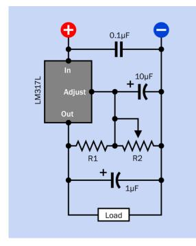
**Figure 19-4.** Schematic for the LM317L adjustable voltage regulator, based on a circuit recommended by National Semiconductor, with bypass capacitors added for ripple rejection.
