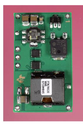
**Figure 17-9.** Another adjustable DC-DC converter. The output voltage is determined by adding an external resistor or trimmer potentiometer. External smoothing capacitors are required, as shown in the component's datasheet.
