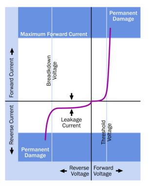
**Figure 26-5.** As the forward voltage across a diode reaches the junction threshold, the diode begins passing current. If the voltage across the diode is reversed, initially a small amount of current leakeage occurs. Excessive forward or reverse voltage will create sufficient current to destroy the component.
