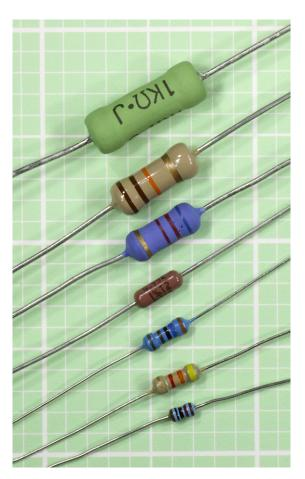
**Figure 10-2.** A range of typical resistors. See text for details.
