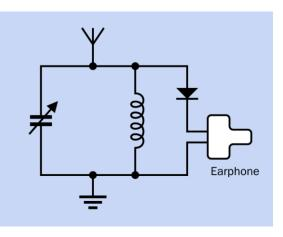
**Figure 13-6.** The principle of an LC circuit is used here in a basic circuit that can tune in to a radio station and create barely audible sound through the earphone at right, using only the broadcast signal for power. The variable capacitor adjusts the frequency of the circuit to resonate with the carrier wave of the radio signal.
