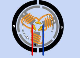
**Figure 22-2.** Three sequential views of a typical three-coil DC motor viewed from the end of its shaft (the shaft itself is not shown). Magnetic effects cause the rotor to turn, which switches the current to the coils via the commutator at the center.
