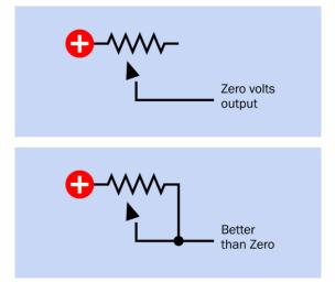
**Figure 11-12.** If the wiper of a potentiometer breaks (indicated by the loose arrow head) as a result of wear and tear, and the potentiometer is being used as a variable resistor, the voltage from it will drop to zero (top schematic) unless the wiper has been tied to one end of the track (bottom schematic).
