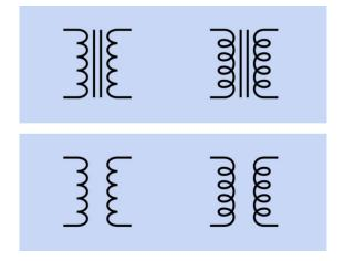
**Figure 15-2.** Alternate symbols for a transformer with a ferromagnetic core (top) and air core (bottom). The differing coil symbols at left and right are functionally identical.
