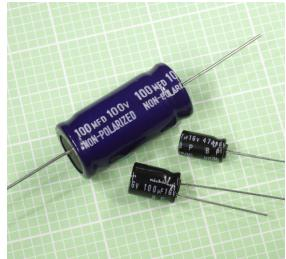
**Figure 12-13.** Bipolar electrolytic capacitors. The larger size of the one at top-left is a consequence of its higher voltage rating. "BP" on the other two capacitors is an acronym for "bipolar," meaning that they have no polarity, even though one lead may be shorter than the other.
