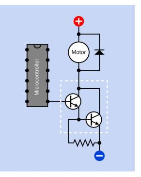
**Figure 28-8.** Where the emitter of one NPN transistor is coupled to the base of another, they form a Darlington pair (identified by the dashed rectangle in this schematic). Multiplying the gain of the first transistor by the gain of the second gives the total gain of the pair.
