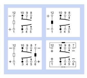
**Figure 9-6.** Relay pinouts depicted in the style commonly found in manufacturers' datasheets, showing different relay types. Top-left: Single coil, nonlatching. Top-right: Single coil, latching. Bottom left: Two-coil, latching. Bottom right: Two-coil, latching, alternate pinouts. (Adapted from a Panasonic datasheet.)
