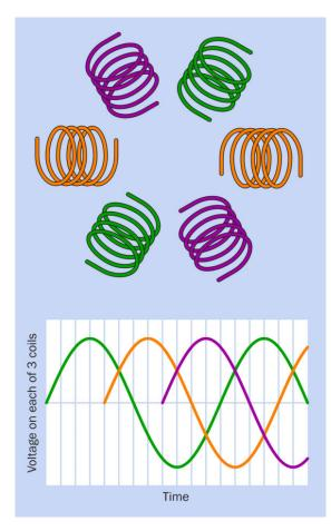
**Figure 23-11.** The graph shows voltage delivered via three wires constituting a three-phase power supply. (The curve colors are arbitrary.) A three-phase motor contains a multiple of three coils—often six, as shown here diagrammatically. The three wires of the power supply are connected directly to the coils, which induce a rotating magnetic field.
