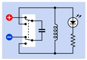
**Figure 13-5.** In this imaginary circuit, the capacitor is charged through the double-pole switch in its upper position. When the switch is turned, the capacitor forms an LC (inductance-capacitance) circuit with the coil, and resonates at a frequency determined by their values. In reality, extremely high values would be needed to obtain a visible result from the LED.
