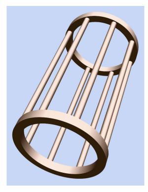
**Figure 23-4.** The rotor of a typical AC motor contains a cage of aluminum (or sometimes copper) in which eddy currents occur, as a result of the rotating magnetic field inside the steel body of the rotor (which is omitted here for clarity). These currents cause their own magnetic fields, which interact with the fields generated by coils in the stator.
