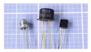
**Figure 27-3.** The unijunction transistors at left and center are becoming obsolete; the one at the right is a programmable unijunction transistor (PUT), still readily available and widely used as a thyristor trigger.
