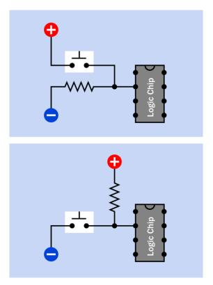
**Figure 10-17.** A pulldown resistor (top) or pullup resistor (bottom) prevents an input pin on a logic chip or microcontroller from "floating" in an indeterminate state when the button is not being pressed.
