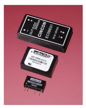
Figure 17-7. A selection of sealed DC-DC converters.
