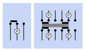
**Figure 5-6.** Left: schematic symbol for a simple SPDT slide pushbutton, where a movable contact shorts together either the left pair or right pair of fixed contacts. Right: A 4PDT pushbutton in which the same principle has been extended. The movable contacts are attached to each other mechanically by an insulator. Each pole terminal is marked with a P.
