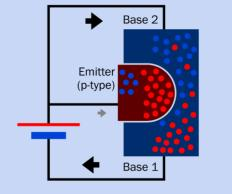
Figure 27-4. Internal workings of a unijunction transistor.
