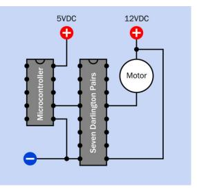
**Figure 28-11.** A chip such as the ULN2003 contains seven Darlington pairs. It will sink current from the device it is driving. See text for details.
