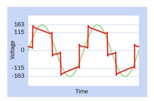
**Figure 18-6.** A cheaply made inverter can generate a distorted wave form that is even higher in noise than a pure square wave. This sample is adapted from an actual oscilloscope trace.
