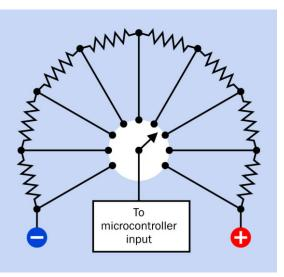
**Figure 7-8.** A resistor ladder can be formed around the contacts of a rotary switch, with the pole of the switch connected to a microcontroller that has an analog-digital converter built in. The microcontroller converts the voltage input to an internal digital value. Thus, one pin can sense as many as twelve input states.
