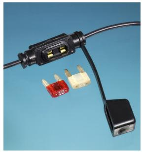
**Figure 4-6.** Two blade-type fuses, commonly used for automotive applications, shown with an inline fuse holder. The plastic cap, at right, is closed over the holder when a fuse has been installed.
