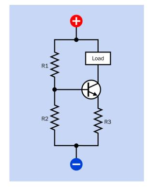
**Figure 28-3.** Resistors R1 and R2 establish a voltage divider to apply acceptable bias to the base of an NPN transistor.
