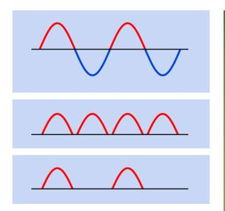
**Figure 26-10.** Top: The voltage-amplitude sinewave of an alternating current source that fluctuates between positive voltage (shown red) and negative voltage (shown blue) relative to a neutral (black) baseline. Center: AC current converted by a full-wave rectifier. Because the diodes do not conduct below their threshold voltage, small gaps appear between pulses. Bottom: Output from a half-wave rectifier.
