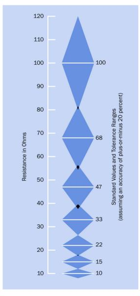
**Figure 10-8.** Graphical representation of standard resistor values (white lines) established by the International Electrotechnical Commission, showing the acceptable range of actual values (dark blue areas) assuming precision of plus-or-minus 20%. The overlap, if any, between each range and the next is shown in black.
