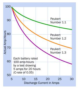
**Figure 2-12.** Actual amp-hour performance that should be expected from three batteries of Peukert numbers 1.1, 1.2, and 1.3 when they discharge currents ranging from 5 to 30 amps, assuming that the manufacturer has rated each battery at 100Ah using the modern system, which usually entails a 20-hour test (a C-rate of 0.05).
