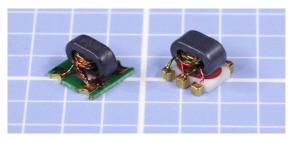
**Figure 15-13.** Two surface-mount transformers, each measuring less than 0.2" square, typically used in communications equipment and suited for frequencies higher than 5 MHz.
