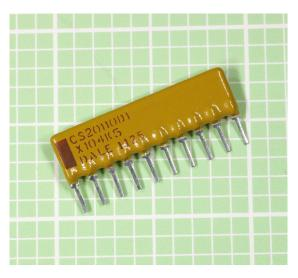
Figure 12-10. A capacitor array in through-hole, SIP format.
