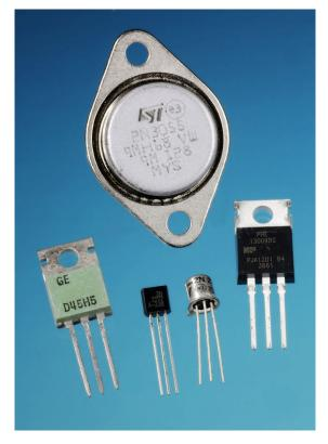
**Figure 28-4.** Samples of commonly used transistors. See text for details.
