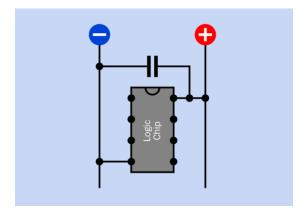
**Figure 12-19.** A bypass capacitor (typically  $0.1\mu$ F) configured to protect an integrated circuit logic chip from voltage spikes and noise in the power supply.
