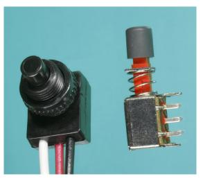
**Figure 5-10.** At right, a simple DPDT latching pushbutton with lockdown. At left, this pushbutton cycles through four states, one of them an "off" state, the others connecting a different pair of its wires in turn.
