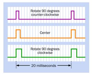
**Figure 24-4.** The turn angle of a small RC servo motor is determined by a pulse width from a controller ranging from 1ms to 2ms in duration. The frequency of the pulses is constant at 50Hz.
