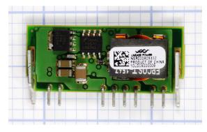
Figure 17-10. Another adjustable DC-DC converter. The output voltage is determined by adding an external resistor or trimmer potentiometer. External smoothing capacitors are required, as shown in the component's datasheet.
