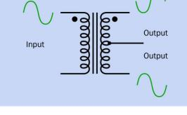
**Figure 15-7.** A dot indicates the start of each winding. Where primary and secondary windings are in the same direction, the voltage output will be 180 degrees out of phase with the input. Where the dots indicate windings in opposite directions, the voltage output will have the same phase as the input. Where a center tap on the secondary winding serves as a common ground, the voltages at opposite ends of the secondary winding will be opposite to each other in phase.
