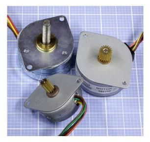
Figure 25-1. Three small stepper motors.
