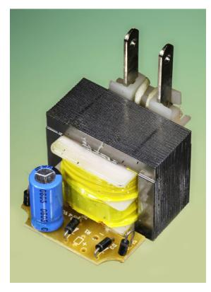
**Figure 16-3.** A relatively old, cheap AC adapter contains only the most rudimentary set of components, and does not supply the kind of properly regulated DC power required by electronic equipment.
