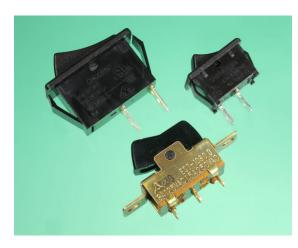
**Figure 6-6.** Three rocker switches, the upper two designed for push-insertion into a suitably sized rectangular hole in a panel. The switch at front-center is intended to be screwed in place, and is more than 20 years old, showing that while the choice of materials has changed, the basic design has not.
