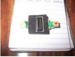
At this point I installed the small ribbon connector into the back of the fingerprint PCB and pushed down the locking tabs to secure it.
