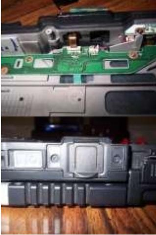
We are almost done now you need to install the ribbon cable protective sheet over the cable to prevent the battery from snagging the cable and tearing it out. Peel the backing tape and stick in on as shown in the picture.
