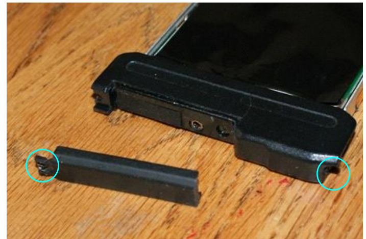
Last would be this piece, not all have it though, Simply snap it into place after the sled is securely In the laptop. Then hold all in place by these two Screw holes.
