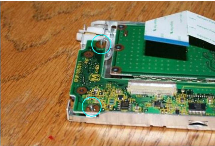
Tighten down two screws here
