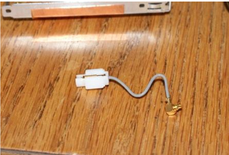
Snap the cable into the plastic piece
